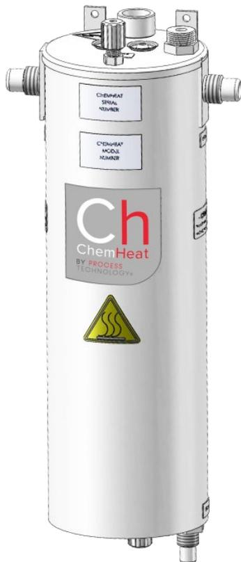
Unique fluid path design and patented purge technology eliminates high-temperature fluid permeation and detects leaks extending product life (MTBF). A low internal volume results in faster heat-up, precise and stable heating performance, lower surface temperatures, and reduced chemistry costs.
